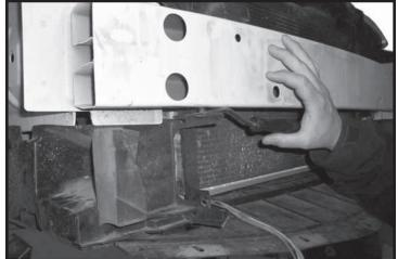
8. Remove plastic filler panel on each side by removing all plastic push fasteners, set panel aside for later notching and reinstallation.
